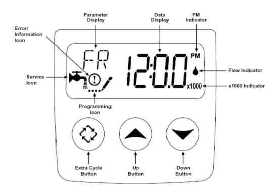
We will first set the time of day to the correct time. Press either the UP or DOWN button and hold for a few seconds. The parameter display will read "TD" (Time of Day) and the "programming" mode icon will appear (4 dots and a pencil). Use the UP and/or DOWN buttons to change the time displayed to the correct time of day. Once the display shows the correct time, press the EXTRA CYCLE button to save your changes.
