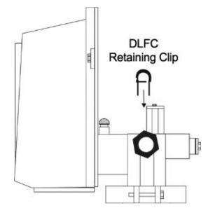
Re-insert the DLFC into the control valve and securely lock into place with the retaining clip when done.
