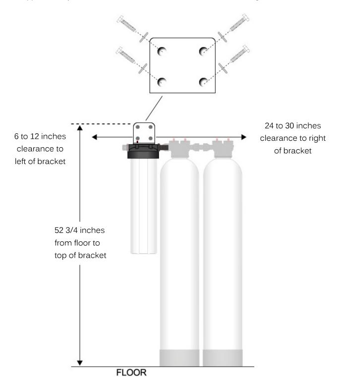
If mounting to drywall, we recommend that you use suitable wall anchors or that you mount a small piece of 3/4 inch plywood to the wall first, ensuring that it is securely screwed into
