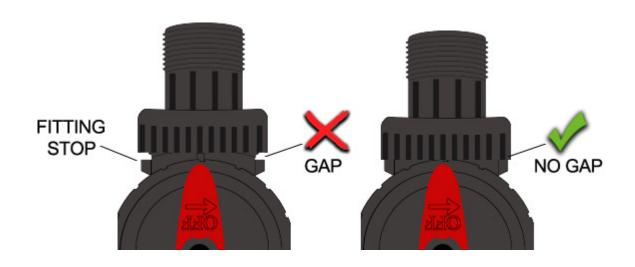
Step 7. - Connect the Bypass Assembly to the ecoTAC™ Valve Head
