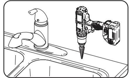
3. Drill a 7/8" hole in the sink using a stepped 7/8" drill bit. If no stepped bit is available, start by drilling a 1/4" hole. Using this hole as a starting point, progressively drill larger holes. Increase drill size by 1/8" until you reach a 7/8" hole.
