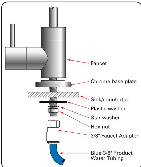
Take length of 3/8" blue tube and make sure it is has a fresh cut and is free of foreign materials and any scratches on the outside surface. Install the tubing into the push in type fitting at the base of the faucet. Make certain that it is inserted all the way in; once inserted give it a slight pull to make sure it is locked into the fitting.
