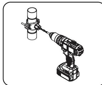
3. For the standard faucets drill a 1/4" hole through one side of the pipe. The drill should be kept straight and centered to avoid damaging the saddle valve. Do not drill through both sides of the pipe!
