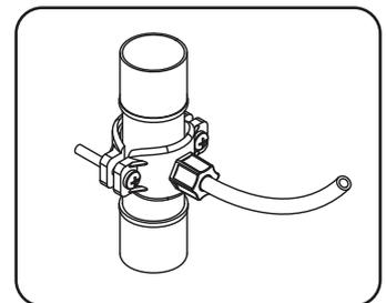
4. Attach 1/4" black tube by slipping the tube through the black compression nut and hand tighten the nut on to the saddle valve.
