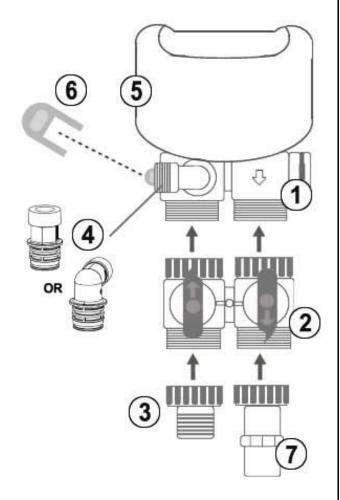
the piping connections and relieves stress on the valve. The 1" NPT connector yokes are connected to the bypass in the same manner (they are normally shipped to you preconnected to the bypass, but you can separate them to make the plumbing to your main water lines easier if you want). Make sure that the connector yoke with the attached flow restrictor is attached to the outlet of the bypass.
