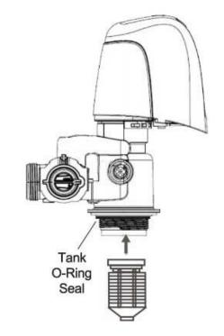
Note: Only use food-grade silicone lubricant. A small bag of lubricant is provided in the small parts bag. Do NOT use petroleum jelly.
