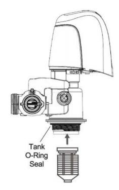
Do NOT use pipe cement ("pipe dope") or Teflon® tape on the threads.
