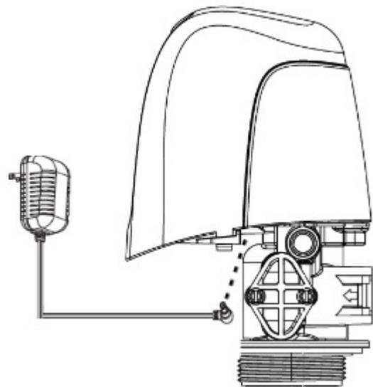
Once plugged in, the touch screen on the control valve will illuminate. The control valve may need to reset to the home position when it is powered up. If it does, the motor will run for a few seconds.
