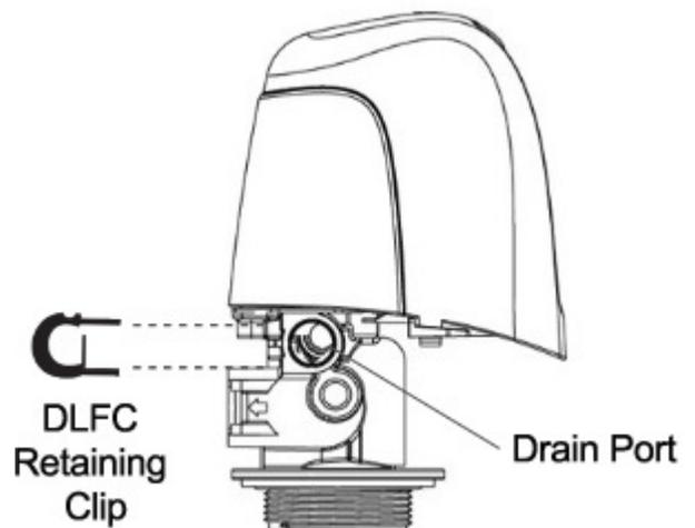
Re-insert the DLFC into the control valve and securely lock into place with the retaining clip when done.
