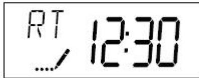
To change the setting, use the UP and DOWN buttons. Press the EXTRA CYCLE button when done. If you do not want to change the current setting, simply press the EXTRA CYCLE button to return to service mode.
