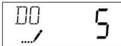
To change the setting, use the UP and DOWN buttons. Press the EXTRA CYCLE button when done. If you do not want to change the current setting, simply press the EXTRA CYCLE button to skip to the next step.
