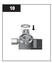
Reinstall the new lubricated orings over the top end of the sleeve.
