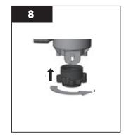
Connect the sleeve bolt at the bottom of the sleeve assembly.
