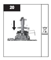
Insert new lamp into chamber and lock into place using a quarter turn clockwise.
