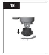
Remove the sleeve bolt at the bottom of the sleeve assembly.
