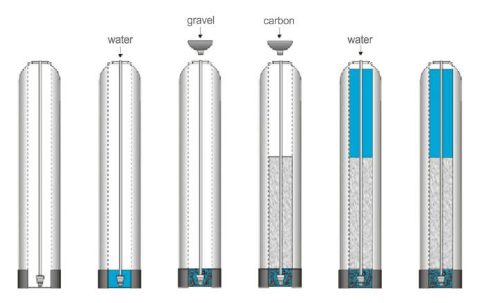
Once this is complete, add the carbon media in the same manner. Use all of the media provided. Depending on the capacity of the system, there will only be enough media to fill the tank to about 1/2 to 3/4 full. This is normal. The media tank should never be filled to the top of the tank as the remaining space, known as the "freeboard," is necessary for the media to have room to expand during the backwash cycle.
