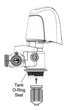
Note: Only use food-grade silicone lubricant. A small bag of lubricant is provided in the small parts bag. Do NOT use petroleum jelly.
