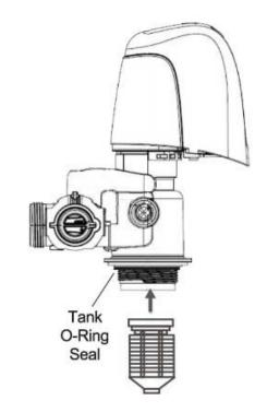
Note: Only use food-grade silicone lubricant. A small tube of lubricant is provided in the small parts bag. Do NOT use petroleum jelly.
