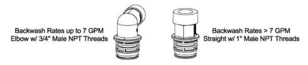
You will need to purchase suitable pipe or tubing for the drain line, either in 3/4 or 1 inch diameter, to match the connection points on the drain line flow control assembly (DLFC). To determine your MINIMUM drain line diameter, look up your model and incoming water temperature using the chart below. If in doubt, match the size of your drain line to the thread size of the DLFC on your control valve.
