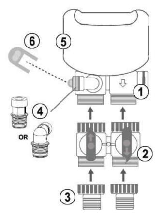
The system's control valve is connected to your incoming and outgoing water lines by way of a
