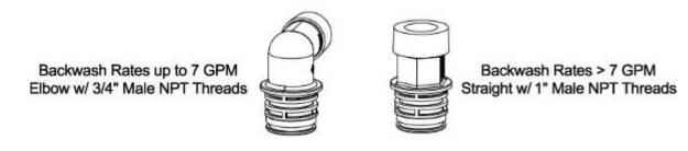
You will need to purchase suitable pipe or tubing for the drain line, either in 3/4 or 1 inch diameter, to match the connection points on the drain line flow control assembly (DLFC). To determine your MINIMUM drain line diameter, look up your model and incoming water temperature using the chart below. If in doubt, match the size of your drain line to the thread size of the DLFC on your control valve.
