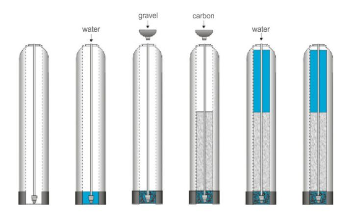
Once this is complete, add the Carbon media in the same manner. Use all of the media provided. Depending on the capacity of the system, there will only be enough media to fill the tank to about 1/2 to 3/4 full. This is normal. The media tank should never be filled to the top of the tank as the remaining space, known as the "freeboard," is necessary for the media to have room to expand during the backwash cycle.
