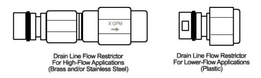
You will need to purchase suitable pipe or tubing for the drain line, either 1/2 or 3/4 inch diameter, to match the connection points on the drain line flow control assembly (DLFC). To determine your MINIMUM drain line diameter, look up your model and incoming water temperature using the chart below. If in doubt, use a 3/4 inch drain line.
