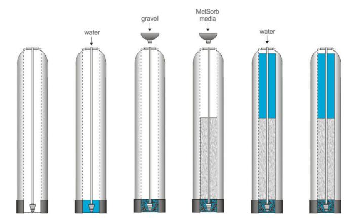
Once this is complete, add the MetSorb media in the same manner. Use all of the media provided. Depending on the capacity of the system, there will only be enough media to fill the tank to about 1/2 to 3/4 full. This is normal. The media tank should never be filled to the top of the tank as the remaining space, known as the "freeboard," is necessary for the media to have room to expand during the backwash cycle.
