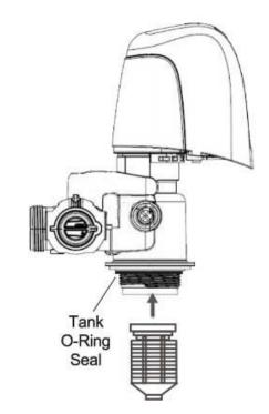
Do <u>NOT</u> use pipe cement ("pipe dope") or Teflon® tape on the threads.
