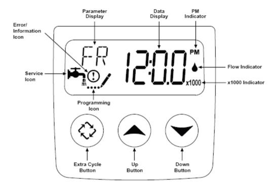
We will first set the time of day to the correct time. Press either the UP or DOWN button and hold for a few seconds. The parameter display will read "TD" (Time of Day) and the "programming" mode icon will appear (4 dots and a pencil). Use the UP and/or DOWN buttons to change the time displayed to the correct time of day. Once the display shows the correct time, press the EXTRA CYCLE button to save your changes.
