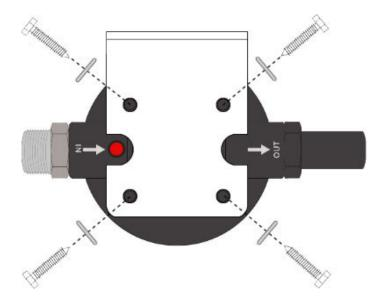
Step 4. - Attach Housing Cap to Wall
