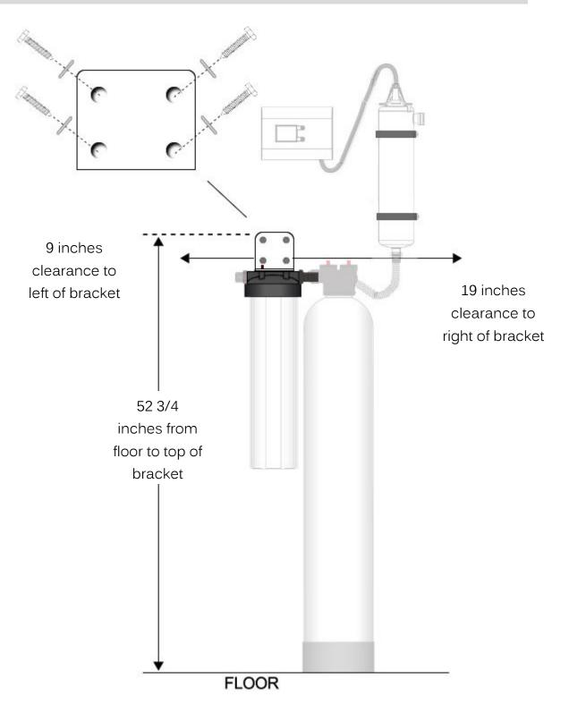
Attach the cartridge filter housing cap and mounting bracket to your wall using the remaining four (4) lag bolts and washers as shown below. The top of the mounting bracket should be mounted EXACTLY 52 3/4 (52.75) inches off the floor. Use a carpenter's
