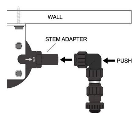
Then, turn the collet to securely lock the fitting.
