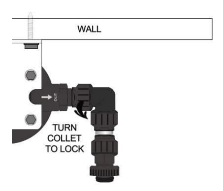
Step 9. - Connect Bypass to Inlet Assembly
