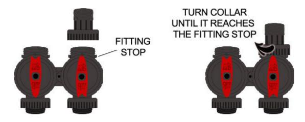
If there is a gap between the outlet adapter's collar and the fitting stop, it is not threaded on far enough. Excessive force is not required to obtain a good seal. Do not over-tighten.
