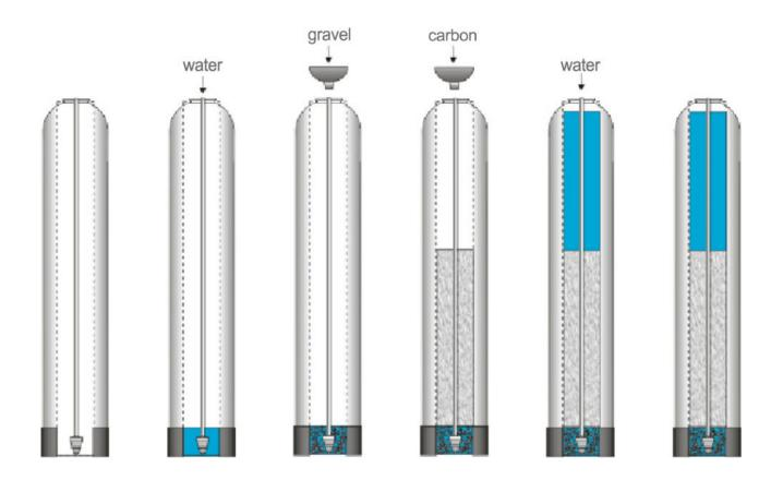
Once this is complete, add the Catalytic Carbon media in the same manner. Use all of the media provided. Depending on the capacity of the system, there will only be enough media to fill the tank to about 1/2 to 3/4 full. This is normal. The media tank should never be filled to the top of the tank as the remaining space, known as the "freeboard," is necessary for the media to have room to expand during the backwash cycle.
