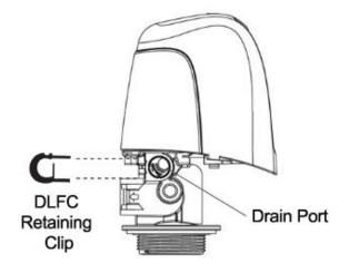
Locate the drain port on the back of your control valve. The drain line flow control assembly (DLFC) is pre-attached to the control valve. For backwash flow rates of 7 GPM or less, the DLFC will be a black plastic housing with 1/2 inch female NPT threads. This housing contains a flow control washer that limits the backwash flow rate. For backwash flow rates exceeding 7 GPM, the DLFC will be a brass adapter with a pre-attached external flow restrictor with 3/4 inch female NPT threads.
