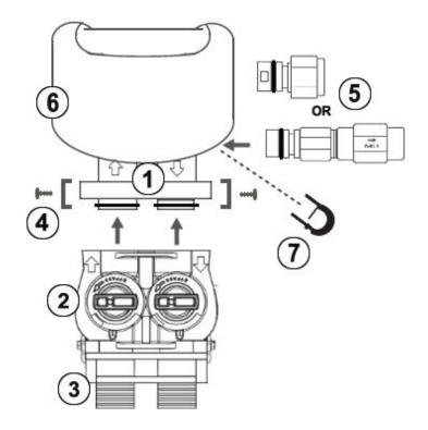
the 1"NPT connector yoke. The 2 piece bypass assembly is secured to the control valve using 2 stainless steel clips. Similarly, the 2 pieces of the bypass assembly, the bypass and the 1" NPT connector yoke, are connected to each other in the same manner (they are
