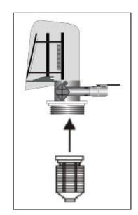
assembly for leverage and do not use tools. A firm grasp with both hands at the base of the valve will work. Do NOT use pipe cement ("pipe dope") or Teflon tape on the valve threads.
