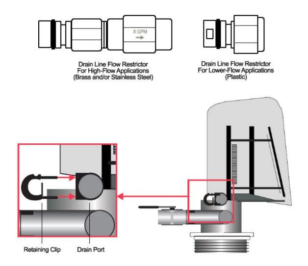
Using an appropriate fitting, connect the NPT threaded outlet of the drain line flow control to your drain line tubing/pipe. You may wish to dry-fit the fitting first to make sure you line up the drain line properly with the drain port on the control valve if you are using rigid pipe.
