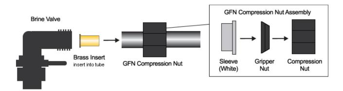
If you have an excessive length of brine line, you should trim it to a more appropriate length first. The brine tubing should be as short and straight as possible. Make sure that the end of the brine tubing is cut square and that the tubing coating is smooth, unmarred, and undamaged. Tighten the black compression nut finger tight, then confirm that there are no kinks or crimps in the brine line.
