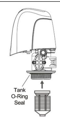
you screw down the valve. The control valve should be hand-tightened (clockwise). Do NOT use the control valve's timer assembly for leverage and do not use tools. A firm grasp with both hands at the base of the valve will work. Do NOT use pipe cement ("pipe dope") or Teflon® tape on the threads.
