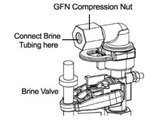
drilled in the brine tank and brine well that you insert the brine tube through to connect it to the brine valve. Feed a small length of brine line through this hole and connect it to the brine valve assembly using a brass insert and the existing plastic GFN compression nut that is attached to the brine valve.
