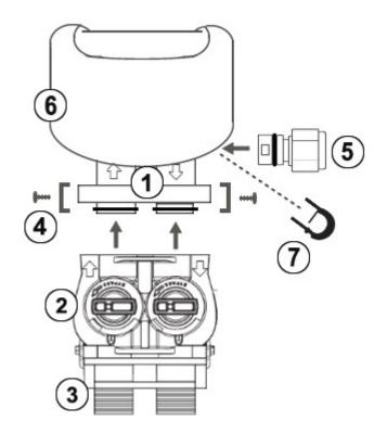
The system's control valve is connected to your incoming and outgoing water lines by way of a bypass assembly with 1"NPT threaded fittings. This assembly is composed of the
