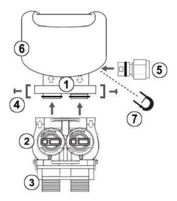
The system's control value is connected to your incoming and outgoing water lines by way of a bypass assembly with 1"NPT threaded fittings. This assembly is composed of the
