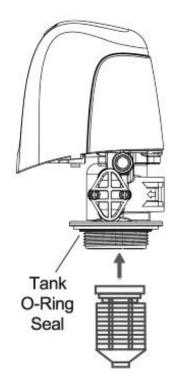
you screw down the valve. The control valve should be hand-tightened (clockwise). Do NOT use the control valve's timer assembly for leverage and do not use tools. A firm grasp with both hands at the base of the valve will work. Do <u>NOT</u> use pipe cement ("pipe dope") or Teflon® tape on the threads.
