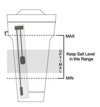
If you have more than 0.3 ppm (mg/l) of iron, and/or more than 0.05 ppm (mg/l) of manganese in your water, we recommend that you use salt with a cleaning additive. Most pellet shaped salts have such an additive. Alternatively, you can add a 4 oz pouch of Pro Products Rust Out (#RO24S) to your brine tank each time you add a bag of salt. This will protect your resin from iron and manganese fouling.
