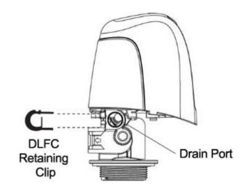
Re-insert the DLFC into the control valve and securely lock into place with the retaining clip when done.
