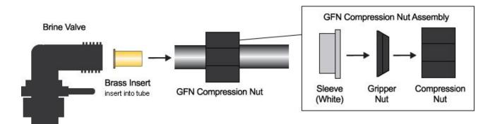
If you have an excessive length of brine line, you should trim it to a more appropriate length first. The brine tubing should be as short and straight as possible. Make sure that the end of the brine tubing is cut square and that the tubing coating is smooth, unmarred, and undamaged. Tighten the black compression nut finger tight, then confirm that there are no kinks or crimps in the brine line.
