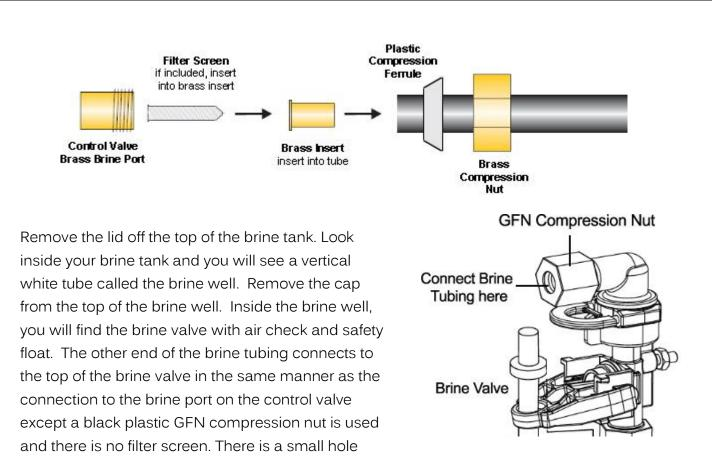
drilled in the brine tank and brine well that you insert the brine tube through to connect it to the brine valve. Feed a small length of brine line through this hole and connect it to the brine valve assembly using a brass insert and the existing plastic GFN compression nut that is attached to the brine valve.
