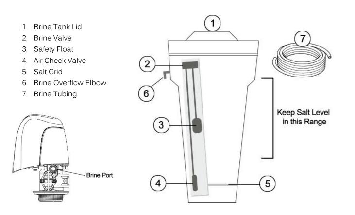
Locate the brass brine port on the right side of your Fleck 5800 control valve (when facing the front of the control valve).
