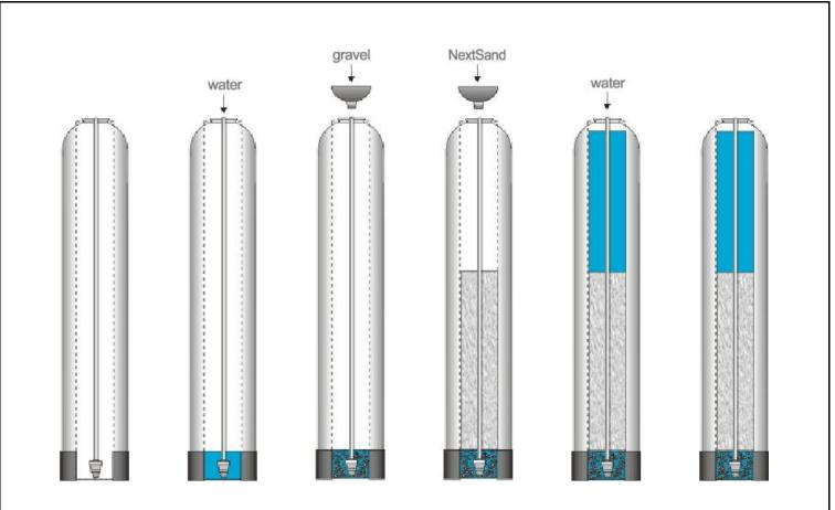
Once this is complete, add the NextSand media in the same manner. Use all of the media provided. Depending on the capacity of the system, there will only be enough media to fill the tank to about 1/2 to 3/4 full. This is normal. The media tank should never be filled to the top of the tank as the remaining space, known as the "freeboard," is necessary for the media to have room to expand during the backwash cycle.
